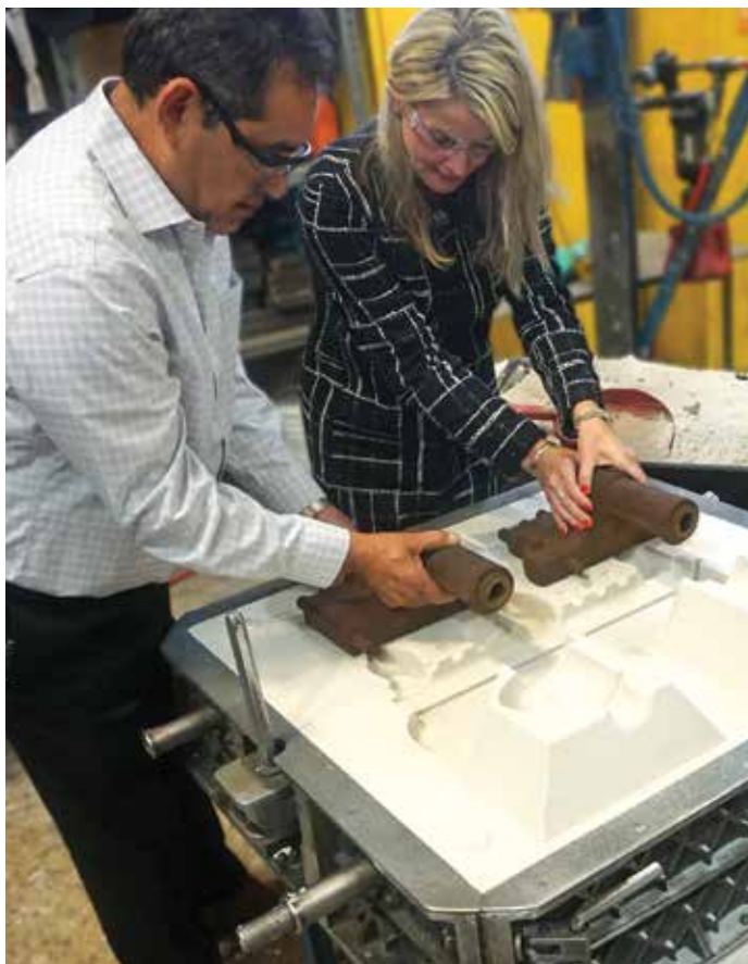
Amanda Torkelson and Alu-Bra's plant superintendent show how a core will be placed into a complex nobake mold.
